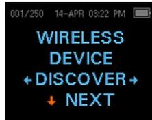
5. Press the DOWN control panel button to advance to other device settings.
